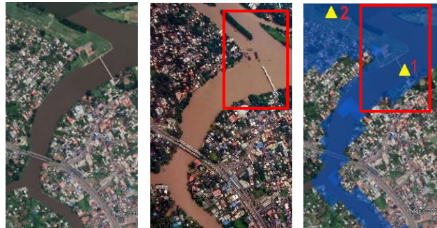
Figure 6. Aerial image of Aluva city on the banks of Periyar river (left); flood extents on 15 th Aug (center) and AIR 100-yr extents in blue on aerial image (right)
